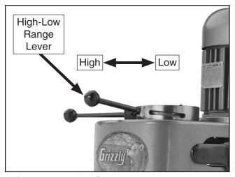
Figure 28. Model G0747 high-low range lever.
